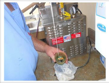
Hold the ring on the vibrator at an angle to reduce trapped air
